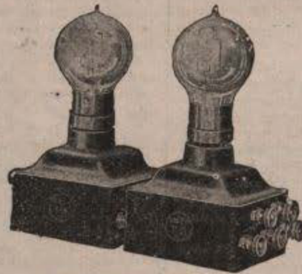
TWO UNIT AMPLIFIERS PLUGGED TOGETHER
